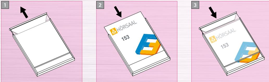
Pull the upper frame edge out of the base panel.
