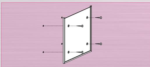
The door sign or the directory is mounted to the wall by four screws\*.
