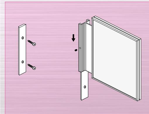
The adapter consists of a mounting base profile and an adapter profile in anodized silver. The base profile is attached to the wall using two screws\*. A grub screw at the side secures the slid over adapter, on which the signs are attached on both sides.
