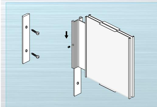
The adapter consists of a mounting base profile and an adapter profile in anodized silver. The base profile is attached to the wall using two screws\*. A grub screw at the side secures the slide over adapter, on which the signs are attached on both sides.
