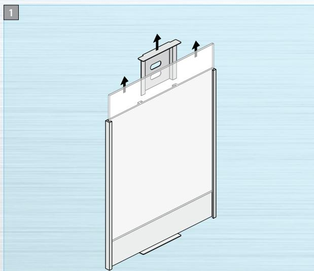
Slide the acrylic cover out of the sign base together with the upper bracket.
