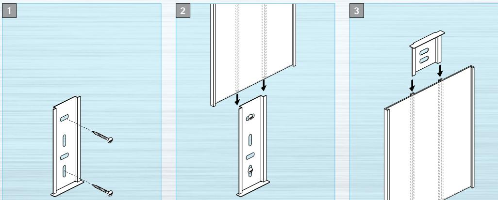
Fasten the lower installation bracket to the wall with two screws\*.
