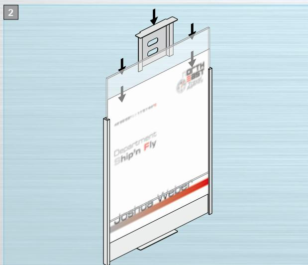
Insert the paper and then fit the acrylic cover and the bracket back in place again.
