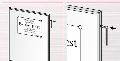
To open the side spring bolts, press in with the Allen key (included in delivery). To prevent it from being opened without authorization, screw the supplied grub screws into the threaded channel.
